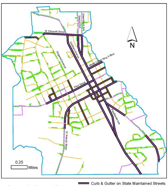
Streets with Curb and Gutter and Stormwater Ditches in the Stormwater Infrastructure Asssessment Project Priority Watershed
